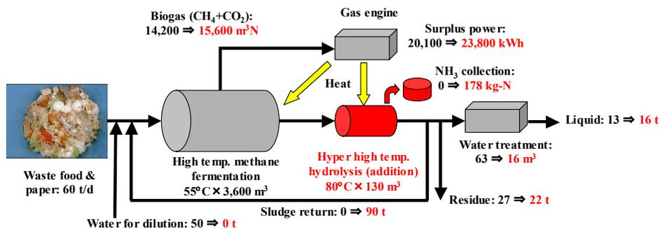
Fig. 4 Flow diagram of dry thermophilic methane fermentation incorporating hyper-thermophillic hydrolysis (prospect in commercial plant, without → with hydrolysis tank)
