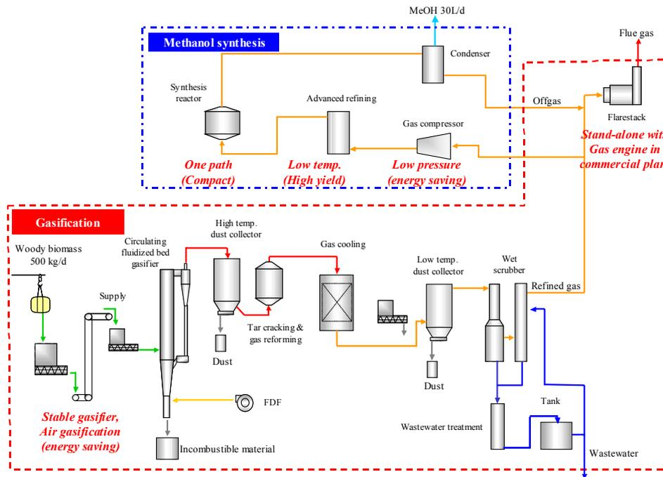
Fig. 3 Flow diagram of gasification and methanol synthesis demonstration
